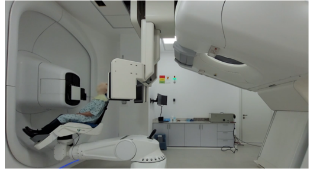
Figure 2: A patient immobilized in a seated position during acquisition of 2 orthogonal 2D X-ray images.
